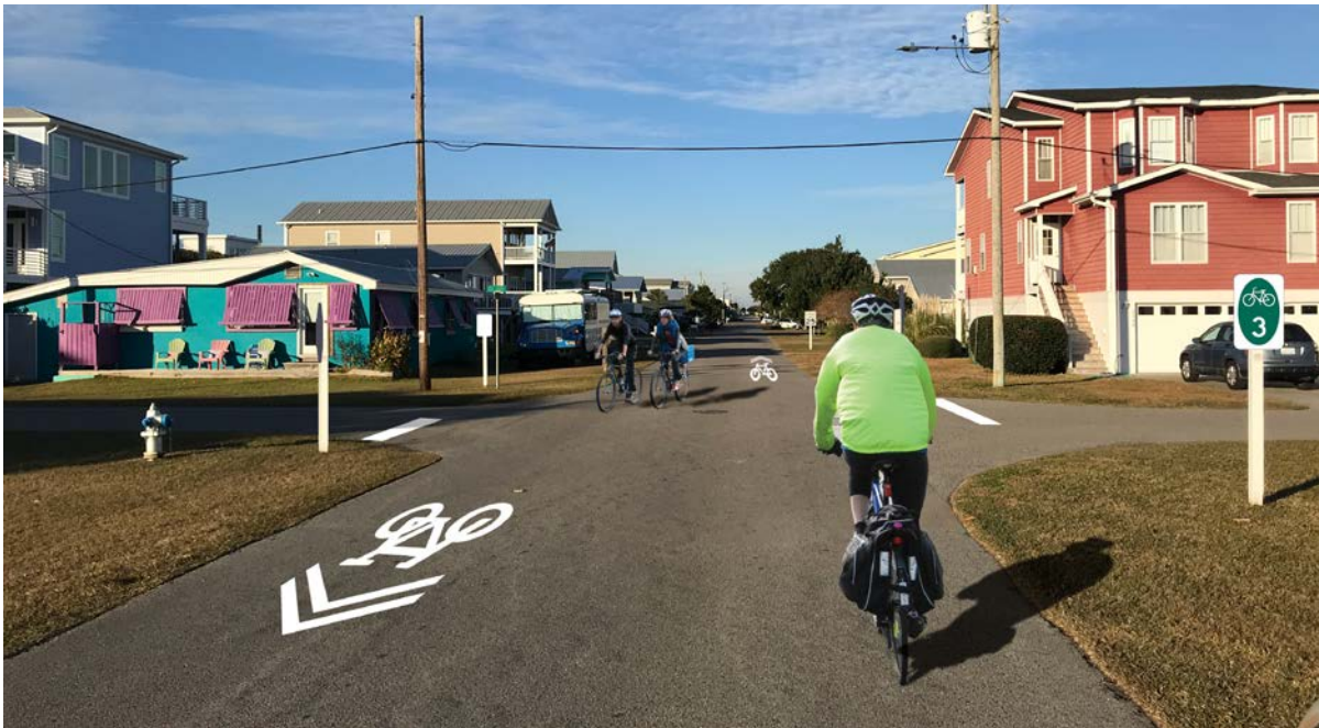
Conceptual image of recommended markings and signage. Note that stop signs and stop bars are flipped in direction to allow for better flow along the bicycle route.
