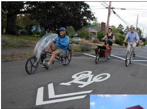
Example of a shared lane marking
