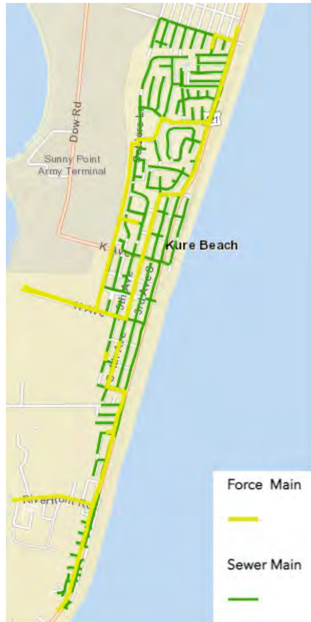
Figure 4.3: Town Wastewater System
