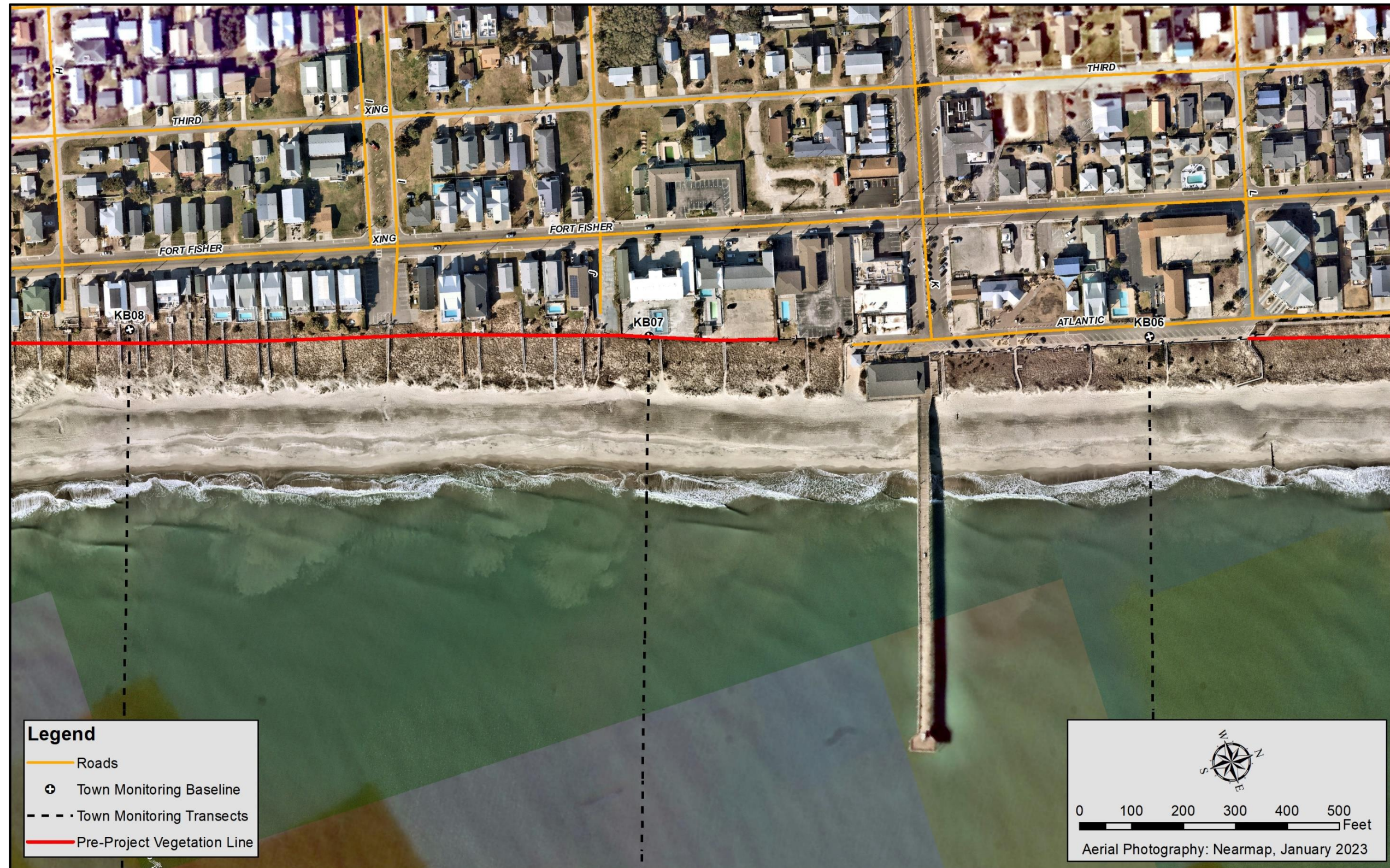
Figure 3-3. Kure Beach Pre-Project Vegetation Line (3 of 6)
